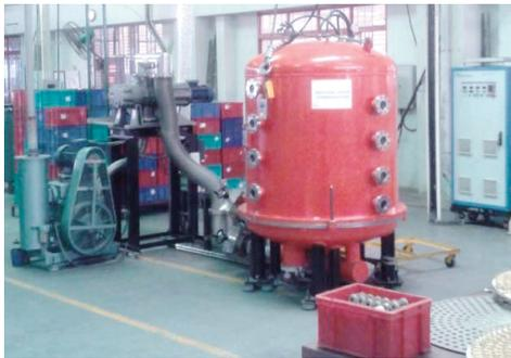
*Industrial scale system to activate brass valves using plasmas for better brass rubber bonding installed in M/S Triton Valves, Mysore*
