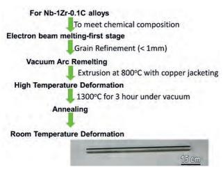
Fig. 6: Flow sheet showing processing of Nb. In the inset fabricated tube is shown.
