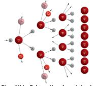
Fig. 1(b): Schematic of sustained and stable fission chain reaction. It is possible with incorporation of suitable absorber materials, which in turn ensure only one neutron enters into fission of next generation
