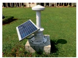
Fig.2: Environmental Radiation Monitor (ERM) of IERMON installed at one of the sites
