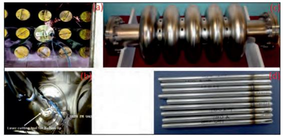
Fig. 5: RRCAT developed Laser based technologies for departmental applications, (a) In situ laser cutting during EMCCR, (b) Bellow lip cutting of TAPS-4, (c) Laser welded 5 cell SCRF niobium cavity (d) Laser welded PFBR fuel pins
