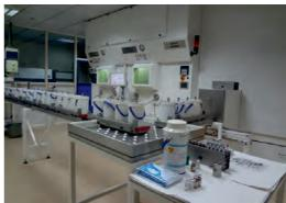
99Mo/99mTc Generator Production Facilities at BRIT (Vashi, Navi Mumbai) -**GELTECH Generator (left) and COLTECH Generator (right)**
