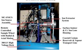
Fig. 5 (i): Multi-Cathode sputter negative ion source
