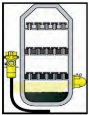
Fig. 3: Radiation-based level measurement by Nucleonic Gauge
