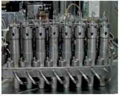
Centrifugal contactors used in CORAL plant
