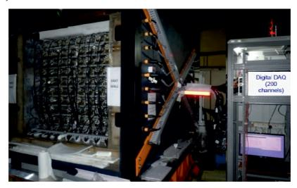
Fig. 7: ISMRAN detector installed inside Dhruva reactor hall for antineutrino measurements
