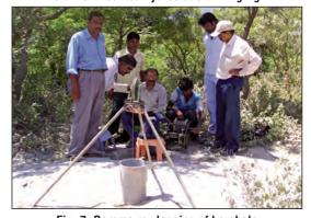
Fig. 7: Gamma ray logging of borehole
