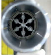
Fig. 10: Dhruva Reactor Fuel Clusters. Left figure shows the overall assembly (3 numbers of them are seen). Right figure shows end view of one of the assemblies. It is a cluster of 7 fuel pins. Dhruva fuel fabrication facilities are more or less identical to those of CIRUS fuel, shown in Fig.9
