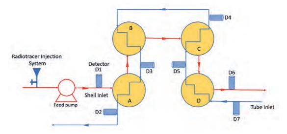
Fig.10: Experimental set-up for Identification of Leaky Heat Exchanger
