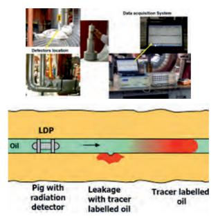
Fig. 9: Leak Detection using Radiotracers
