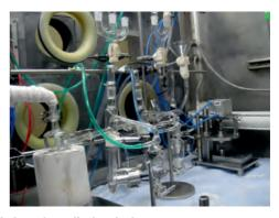
In-cell gadgets inside the lead shielded plants for radiochemical processing of 177Lu (left) and 131 (right)
