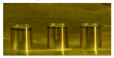
Fig. 7: 60 Co Sealed Sources (CTS) for Teletherapy Machines
