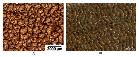
Fig. 4:Typical signature pattern for (a) Single phase FAC (Scallops) and (b) Dual phase FAC (tiger stripe pattern) observed on Indian PHWRs secondary circuit components
