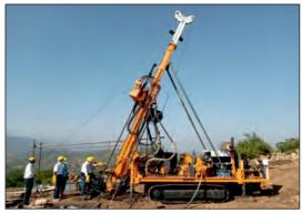
Fig. 5: Sub surface exploration for uranium by crawler mounted hydrostatic drilling rig
