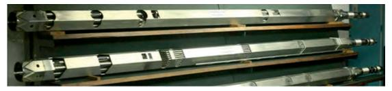
Fig. 12: Fuel assemblies for PFBR. It comprises of several pins each having uranium-plutonium MOX pellets. Since MOX is stable form of uranium and plutonium hence the fuel fabrication is carried directly in air media. However, leak tightness requirements are same as those of carbide fuel for FBTR (see Fig. 11) since radiological safety requirements are same for both. The fabrication is carried out at AFFF, BARC, Tarapur.
