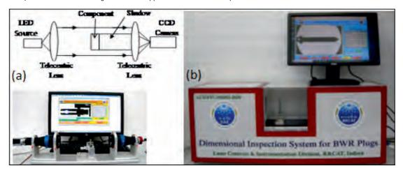
Fig. 8: RRCAT developed nuclear metrology set up, (a) Operating principle, (b) Full System
