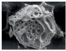
Fig. 16 (b): Grain from a high burn-up PHWR fuel showing fission gas bubbles, channels and metallic fission products. This is as seen in radiation shielded Scanning Electron Microscope (SEM). Grain size is ~ 30 µm
