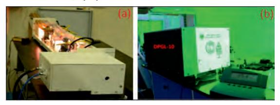
Fig. 2: RRCAT developed (a) Flashlamppumped IRNd:YAG laser and (b) Diode pumped greenNd:YAG laser
