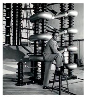
Fig. 2: 1 MV Cockcroft-Walton Accelerator (Cascade Generator) at TIFR, in 1953
