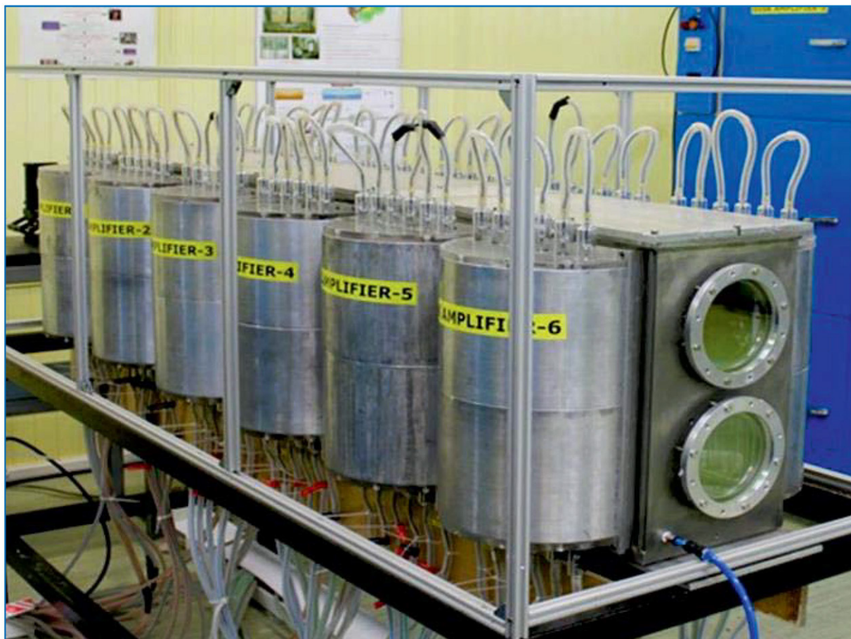
80 J, 10 ns Nd:Glass laser system test bed developed at RRCAT
