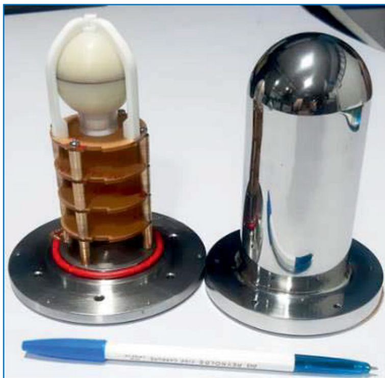
Prototype TEPC Assembly 1.5 Kg full weight
