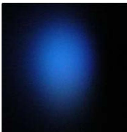
Fig.101. Photograph of blue light emission from thin film of PMMA containing  $\text{ZnGa}_{1.5}\text{In}_{0.5}\text{O}_4$  nanoparticles, on a quartz substrate. The excitation wavelength was 270 nm.
