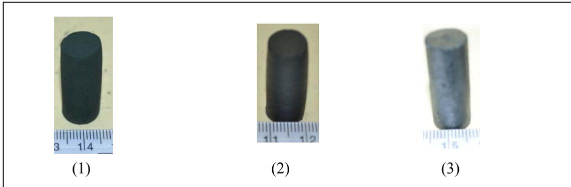
**Fig.5.9 Pictures of pin during various stages of fabrication using mould size pin as mentioned in Table 5.1 Sr. No. 3 : (1) Compacted pin, (2) Sintered pin, and (2) TSMTG pin**
