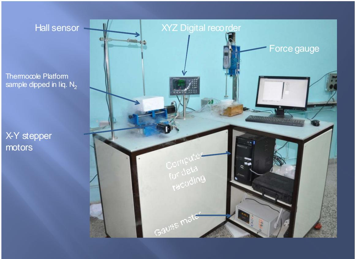
**Fig.2.14 Trapped magnetic field and levitation force measurement system**
