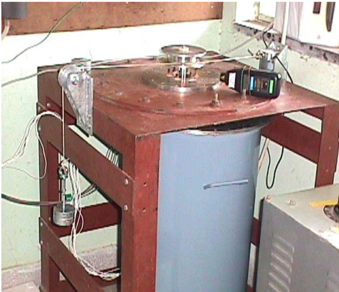
**Fig.A.6 HTSC motor assembly**
