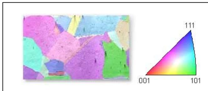
**Fig. 2.11. Inverse pole figure mapping**
