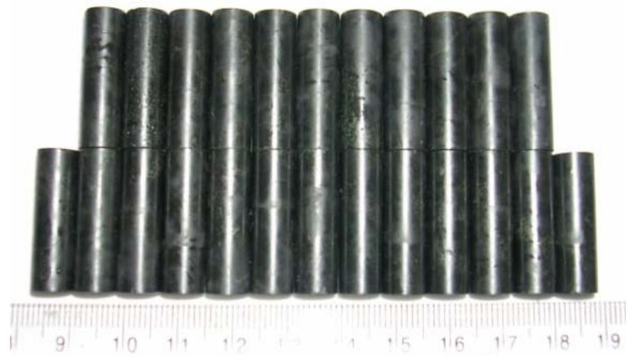
**Fig.5.13 Machined TSMTG pins using composite B (NDR-PI-1)**
