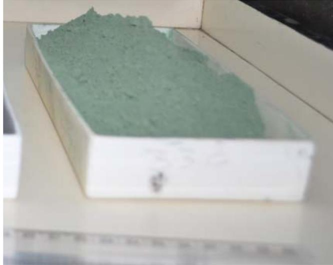
**Fig. 3.4 Y-211 powder (approx 0.5 kg) in an alumina boat**
