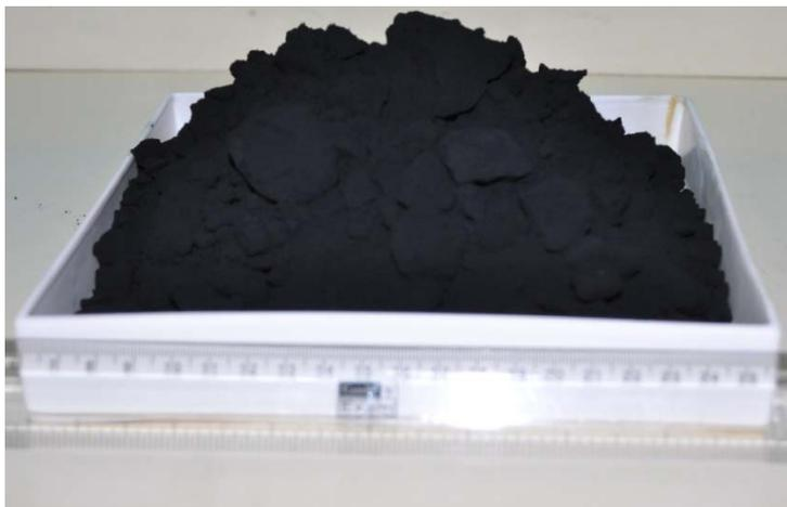
**Fig.3.3 Y-123 powder (approx one kg) in an alumina boat**
