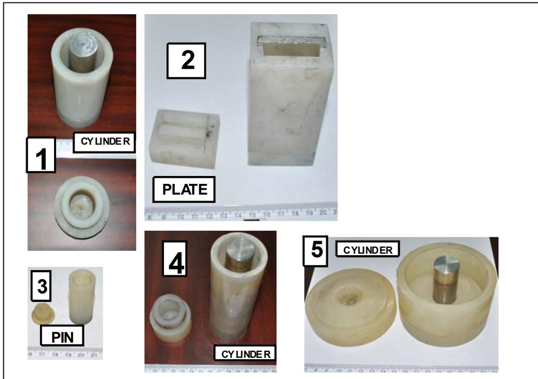
**Fig.5.3** Picture of moulds for fabricating components :- (1)-Mould for hollow cylinder 1, (2)- Mould for Plates, (3)-Moulds for PINS, (4)-Moulds for hollow cylinder 2, (5)-Mould for hollow cylinder 3
