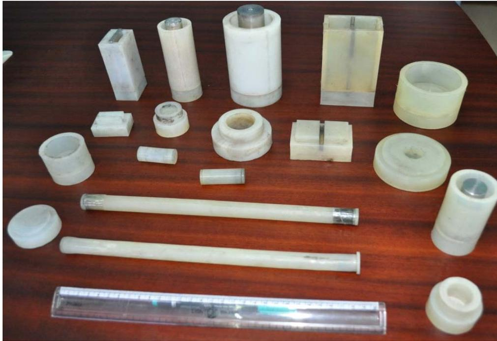
**Fig.5.14 Picture of rubber mould used to fabricate MTG components**
