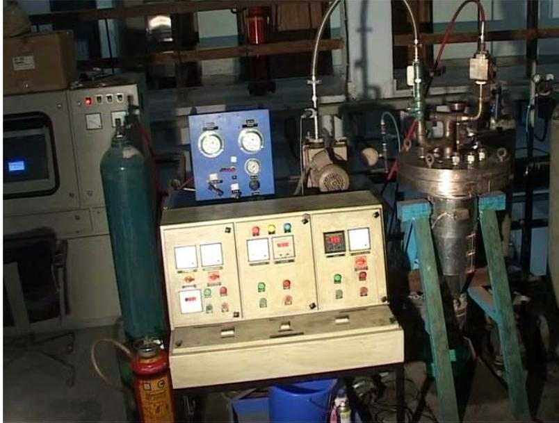
**Fig.3.2: Indigenously fabricated Impregnator Unit**
