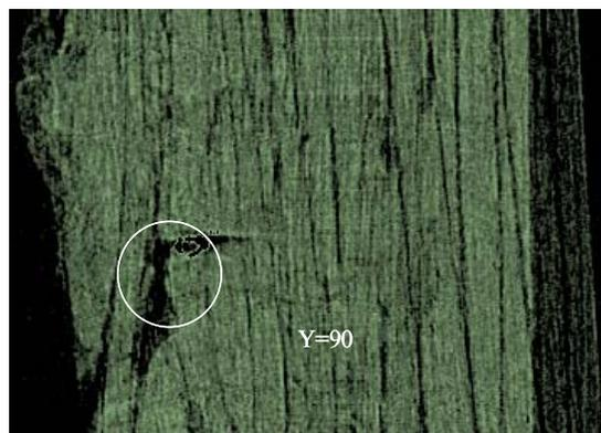
**Fig. 3.15:** Crack propagation in the X direction at different Y planes (specified in each image), due to application of pressure (encircled portion)
