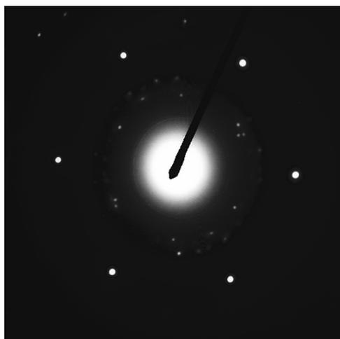
**Fig. 6.7: SAED pattern obtained by aligning the electron beam perpendicular to the plane of a hexagonal nanoplate**
