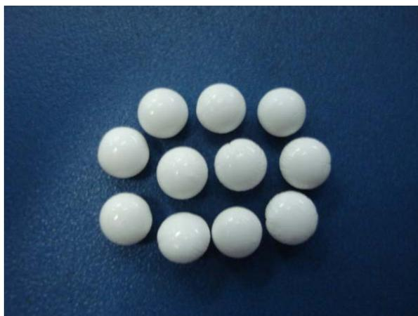
**Fig. 5.10: Typical optical image of the microcapsules**
