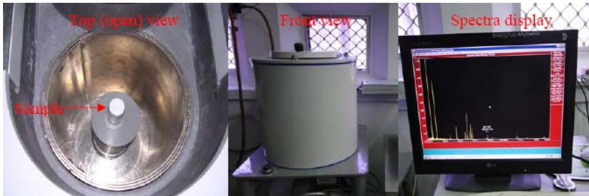
**Figure 2.8 The High-purity germanium detector (HPGe)**
