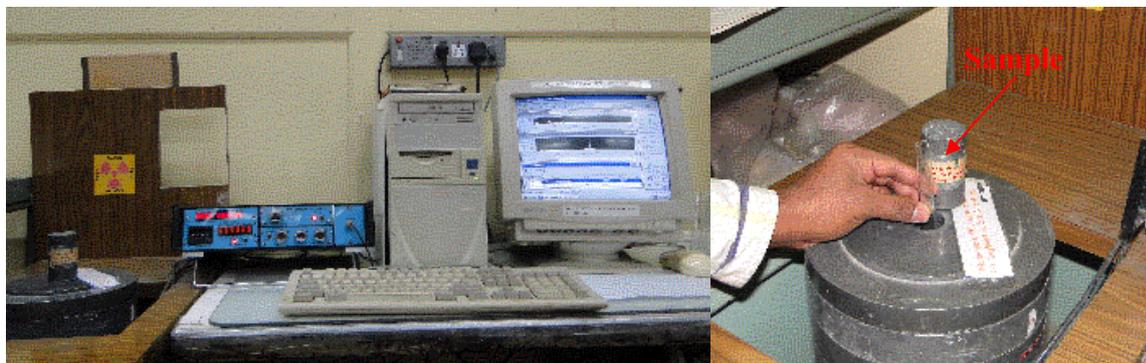
**Figure 2.7 NaI(Tl) detector set-up**
