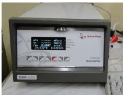
**Figure 2.9 The Anton Paar Viscometer used for the viscosity measurements.**
