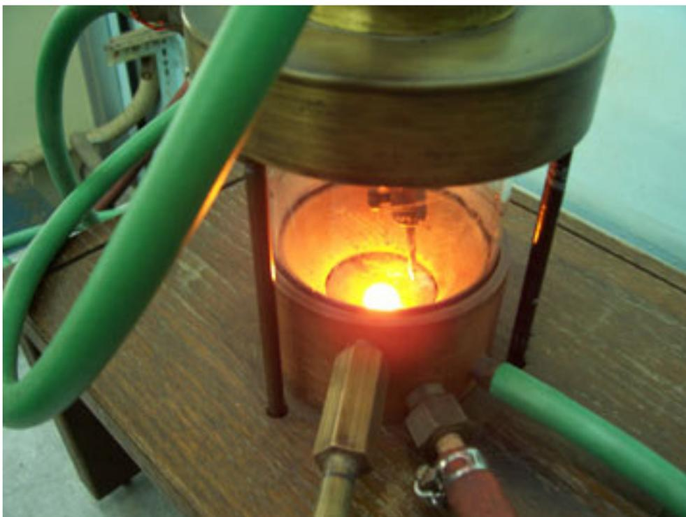
**Fig. 2.1** *The chamber of the arc furnace used during the study*
