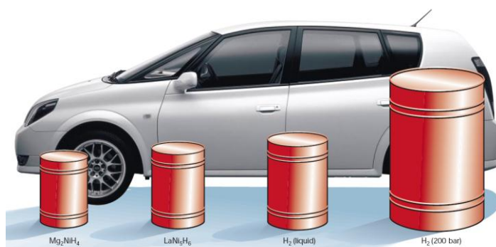
Figure 1.5: Comparison of the size of hydrogen tank with different ways of storage.
