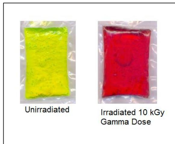
Figure 5.4: Actual photographs of unirradiated and irradiated gel
