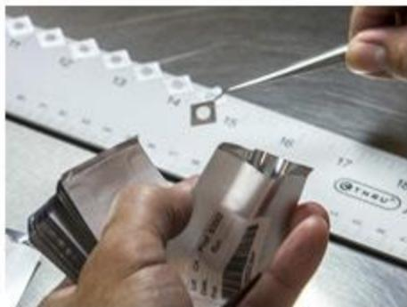
Figure 1.12: Radiochromic film RisoB3 dosimeter
