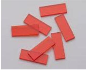
Figure 1.10: Dyed Perspex dosimeters (Harwell Red 4034 Dosimeters (United Kingdom))
