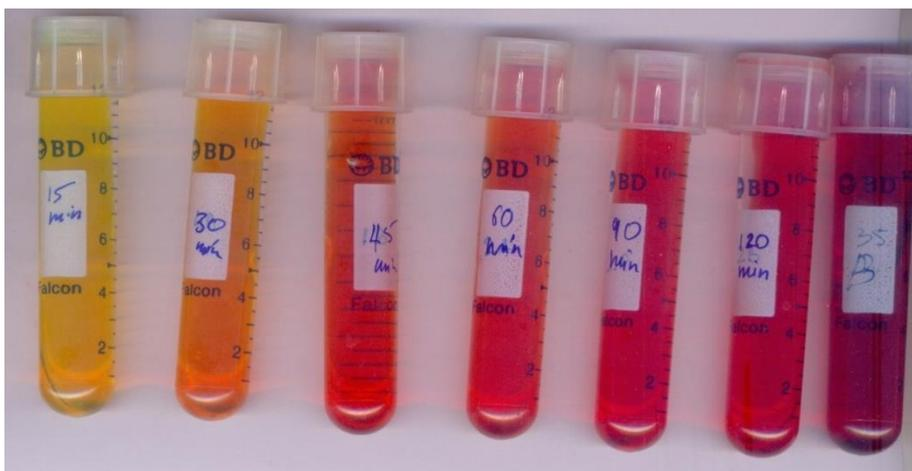
Figure 4.55: Colour development with dose in radiochromic dosimeter
