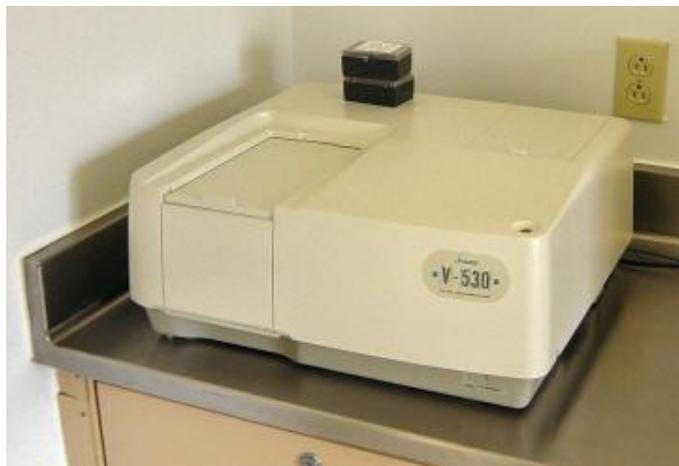
Figure 2.15: Jasco V-530 UV/Vis double beam spectrophotometer
