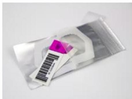
Figure 1.11: Radiochromic film dosimeter
