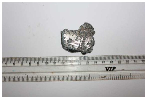
**Fig.6.5** Electrodeposited product obtained from  $\text{NdCl}_3\text{-LiCl-KCl}$  electrolyte.
