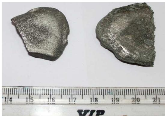
**Fig.6.4** Electrodeposited product obtained from  $\text{PrCl}_3\text{-LiCl-KCl}$  electrolyte.
