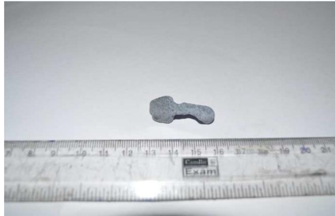
**Fig.7.13** Photograph of the Nd-Fe product obtained in our experiment.
