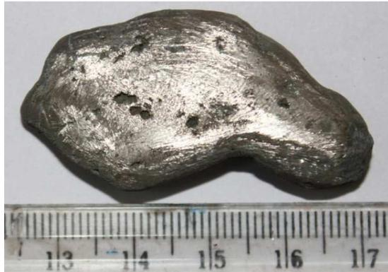
**Fig.6.3** Electrodeposited product obtained from the electrolysis of  $\text{CeCl}_3$  in  $\text{LiCl-KCl}$  flux.
