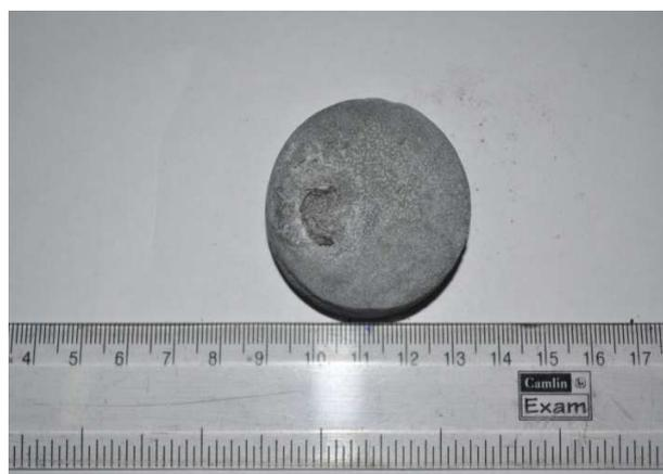
**Fig.6.2** Electrodeposited product obtained from the electrolysis of  $\text{LaCl}_3$  in  $\text{LiCl-KCl}$  flux.
