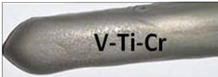
*Fig 4.1.8: V-Ti-Cr alloy finger prepared by aluminothermy process, refined by electron beam melting followed by homogenization by vacuum arc melting*
