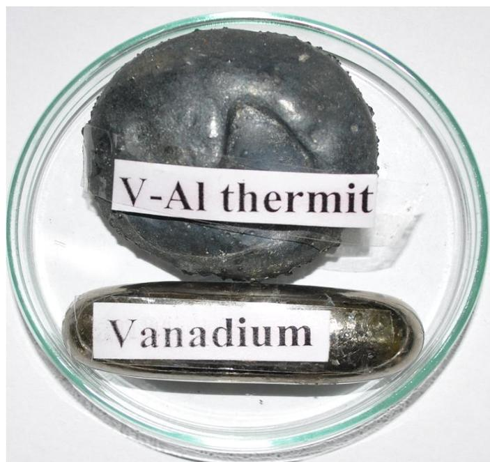
*Fig. 4.1.2: Vanadium-aluminum thermit along with completely refined product vanadium*
