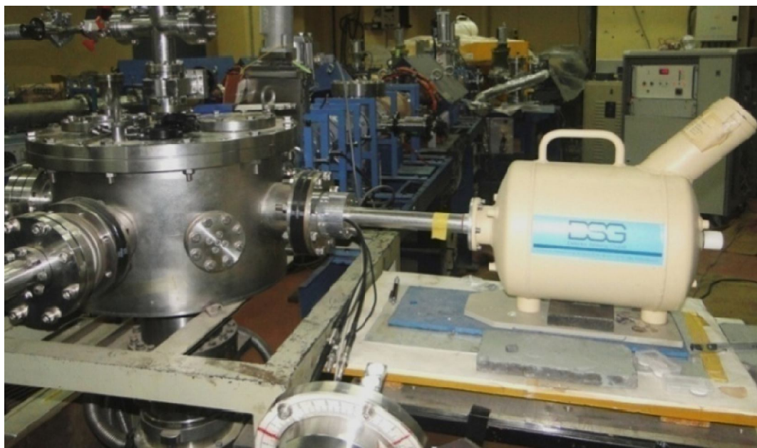
Fig. 2.2: PIGE set up at FOTIA, BARC showing beam chamber and HPGe detector system.
