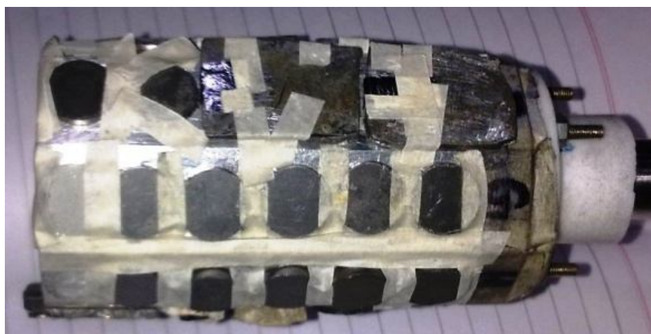
Fig.2.5: Multi-target ladder with targets at IOP, Bhubaneswar
