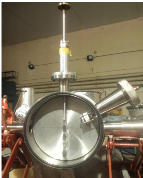
Fig. 2.7: Chamber showing targets mounted on a sample holder for irradiation at BARC-TIFR Pelletron facility.
