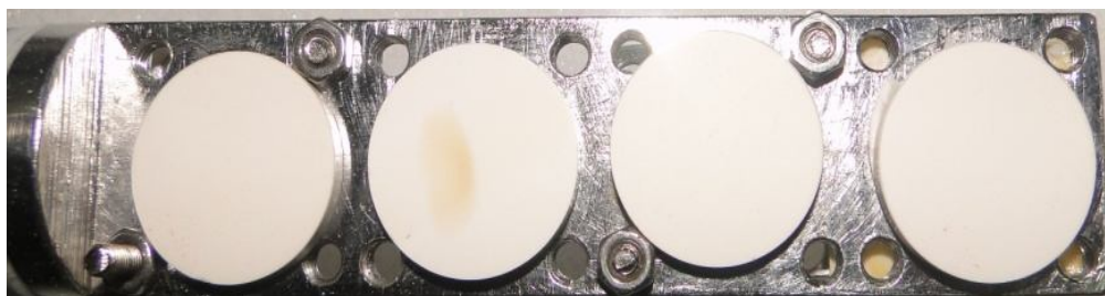
Fig. 2.3: Target ladder at FOTIA, BARC showing mounted targets.
