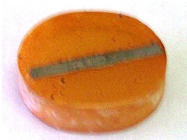
**Fig. 3.1** Photograph of Type 304L NAG 1 specimen mounted in cold setting resin for microstructure evolution.
