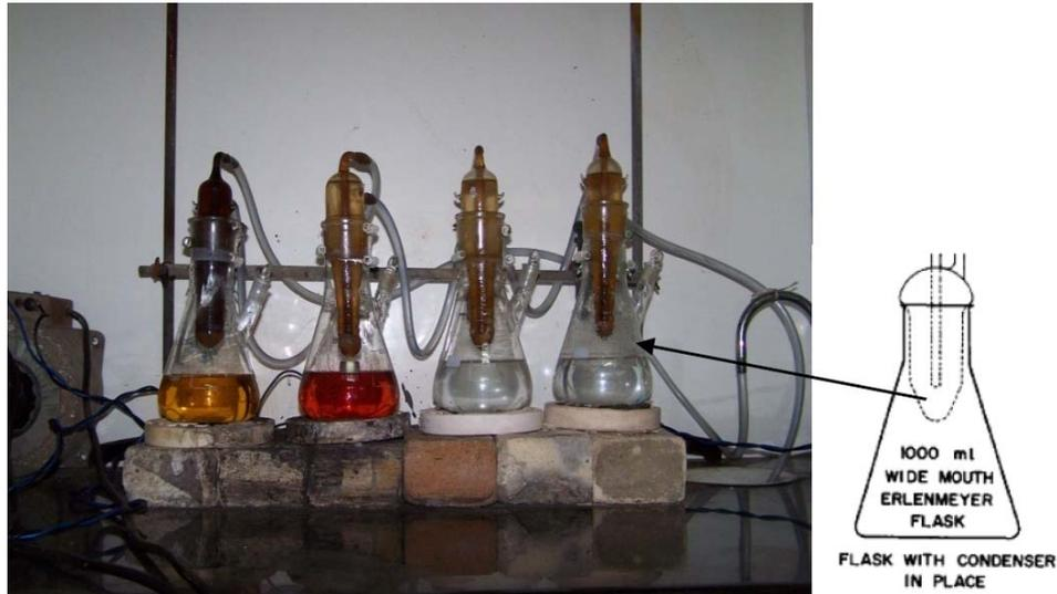
**Fig.3.6** Photograph of the set up used for Practice C, A262, ASTM.
