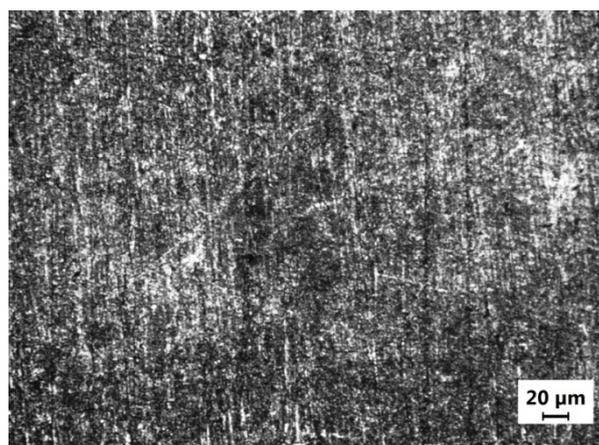
**Fig.5.4** Morphology of corrosion attack (observed by optical microscope) on longitudinal surface of Type 304L2 (ASTM grain size no 4) exposed to near boiling 6M  $HNO_3$  at  $0.93 V_{SCE}$ .
