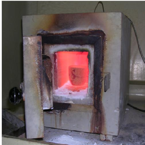
*Fig 3.3. Chamber type furnace used for exposure of specimens with sodium borosilicate melts.*
