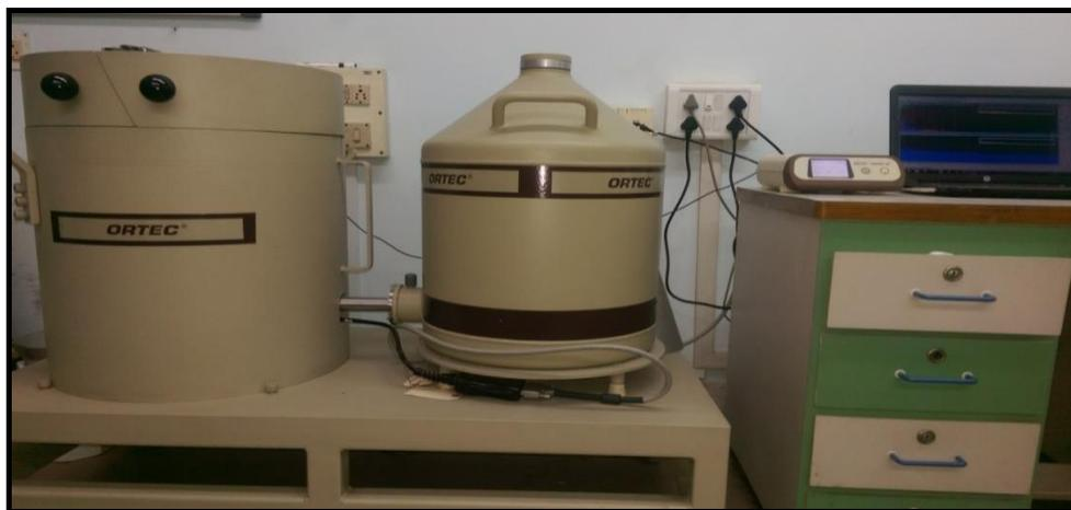
**Figure 3-11: P type HPGe detector assembly with electronics(ORTEC)**
