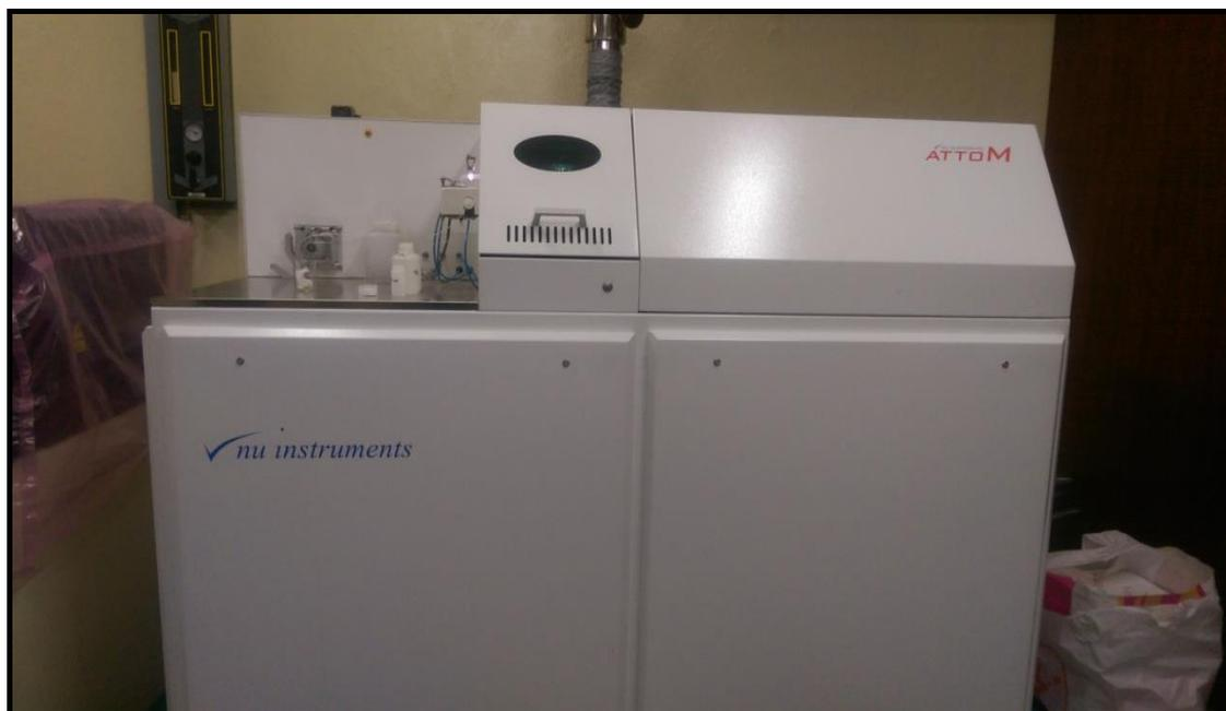
**Figure 3-14: HR-ICP-MS (ATTOM, Nu Instruments, UK)**
