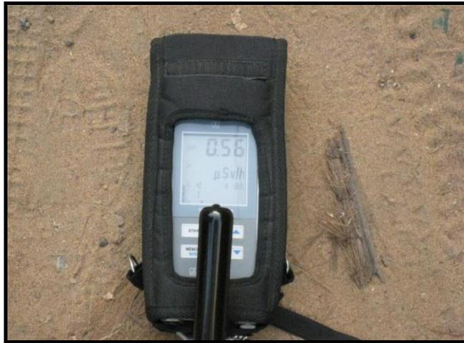
**Figure 3-3: Portable hand-held survey meter (Atomtex 1123)**
