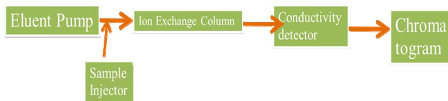
**Figure 2.4: Block diagram for an Ion Chromatography system.**
