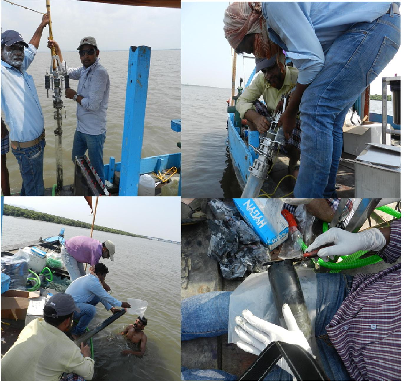
**Figure 3.11:** Collection of core sample using gravity corer
