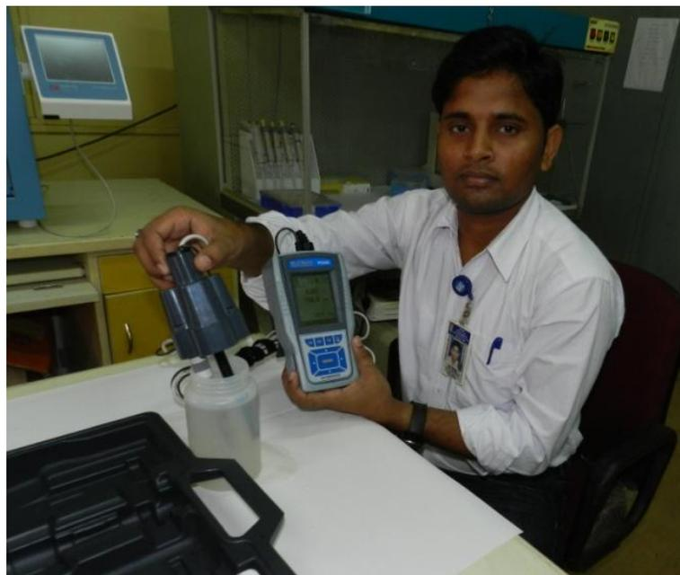
**Figure 3.13:** Multi-parameter kit (EUTECH Instrument PC650)
