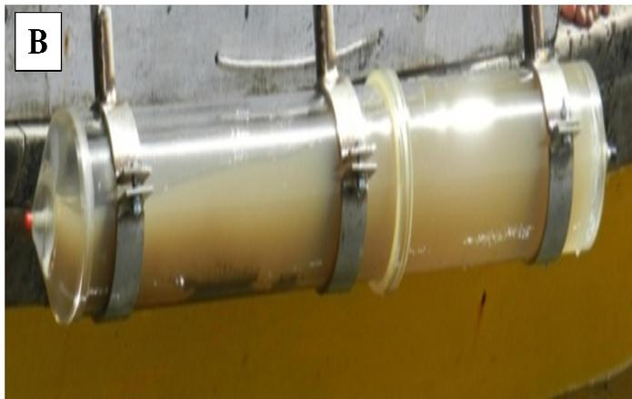
**Figure 3.12:** Deployment of suspended sediment sampler and collection
