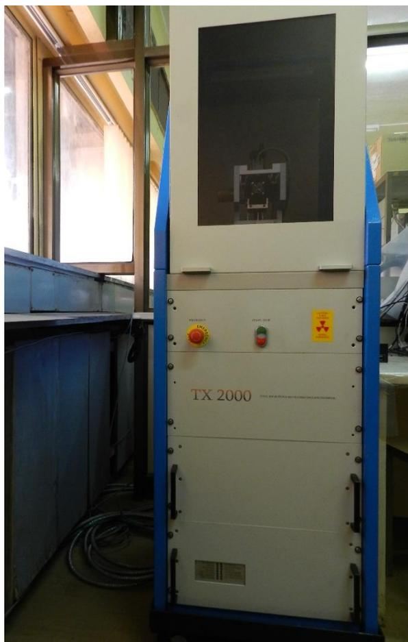
**Figure 2.30:** TX2000 TXRF instrument used in the present study
