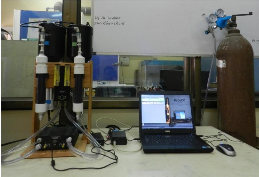
Figure 2.4: The Radium Delayed Coincidence Counter used in the study
