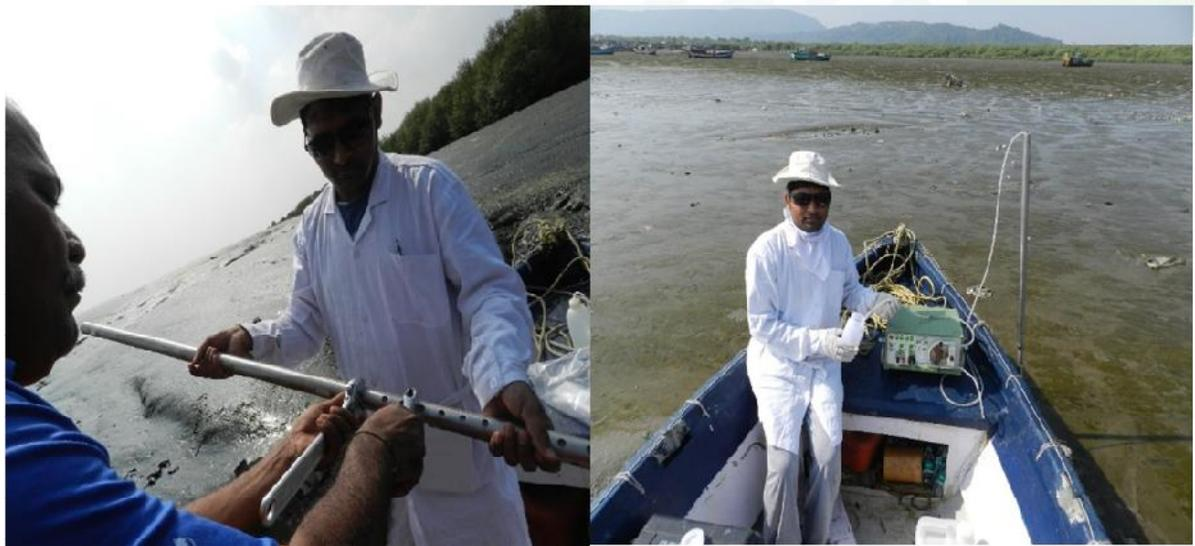
**Figure 3.10:** Piezometer groundwater sampler and groundwater sampling
