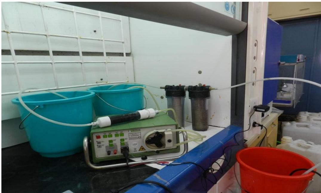
**Figure 3.6:** Radium Pre-concentration on MnO<sub>2</sub> fiber system in the Laboratory
