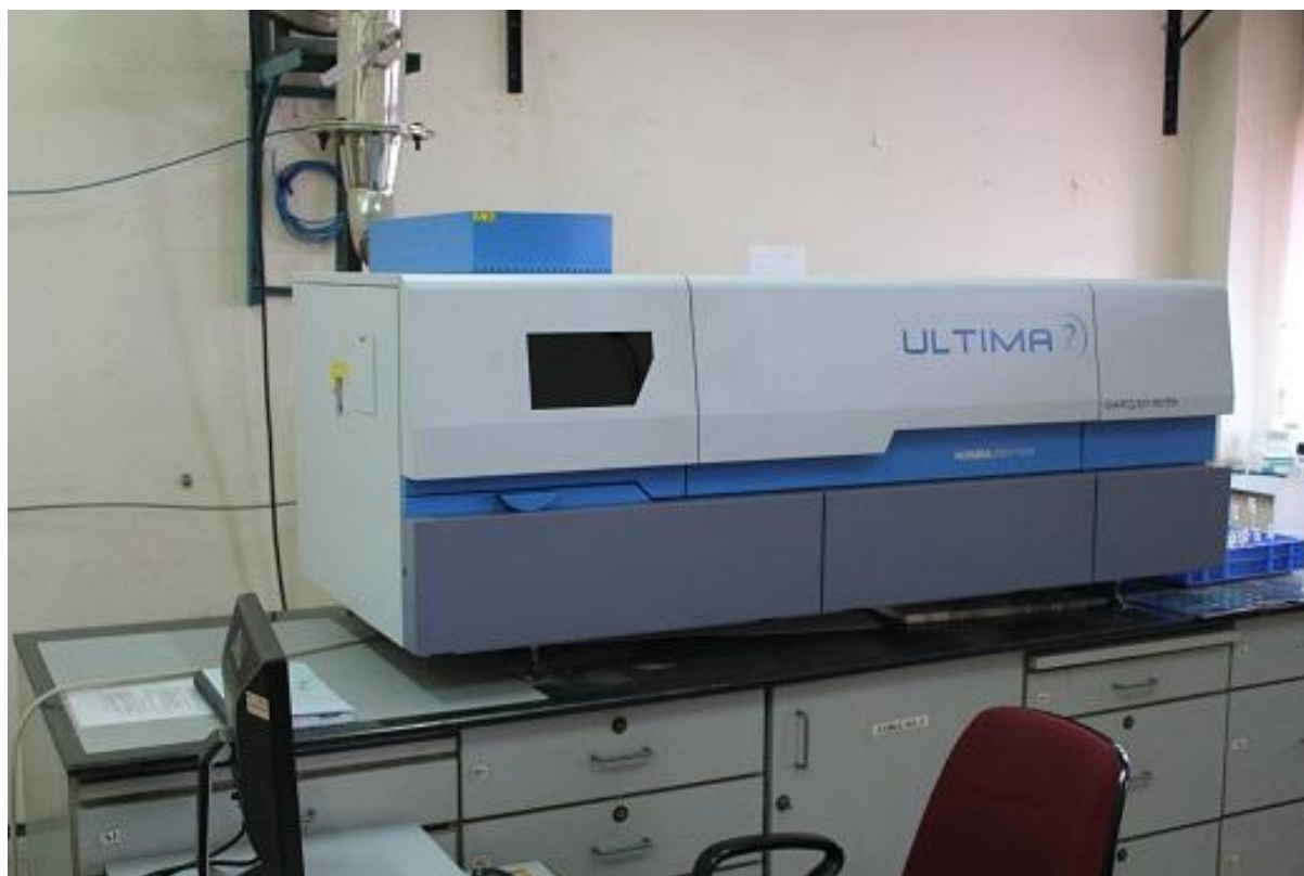
Fig. 2.9 Inductively Coupled Plasma-Atomic Emission Spectroscopy (ICP-AES) employed for the analysis of rare earth elements
