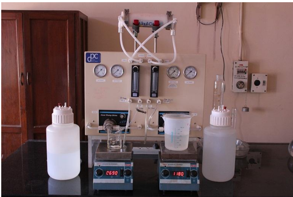
Fig. 2.8 Hollow Fibre Membrane contactor used in the present work
