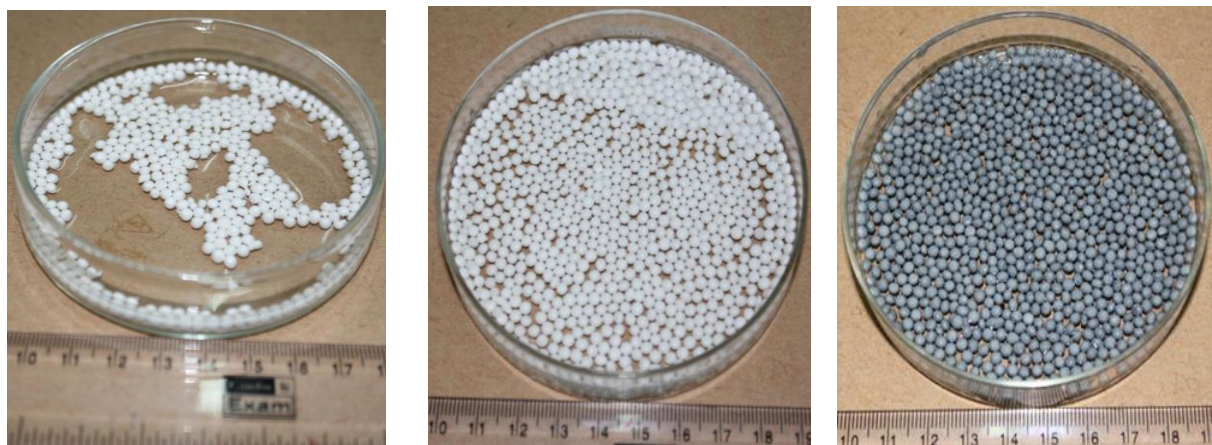
Fig. 3.1 Optical images of PES/D2EHPA, PES/PVA/D2EHPA and PES/PVA/MWCNT/D2EHPA
