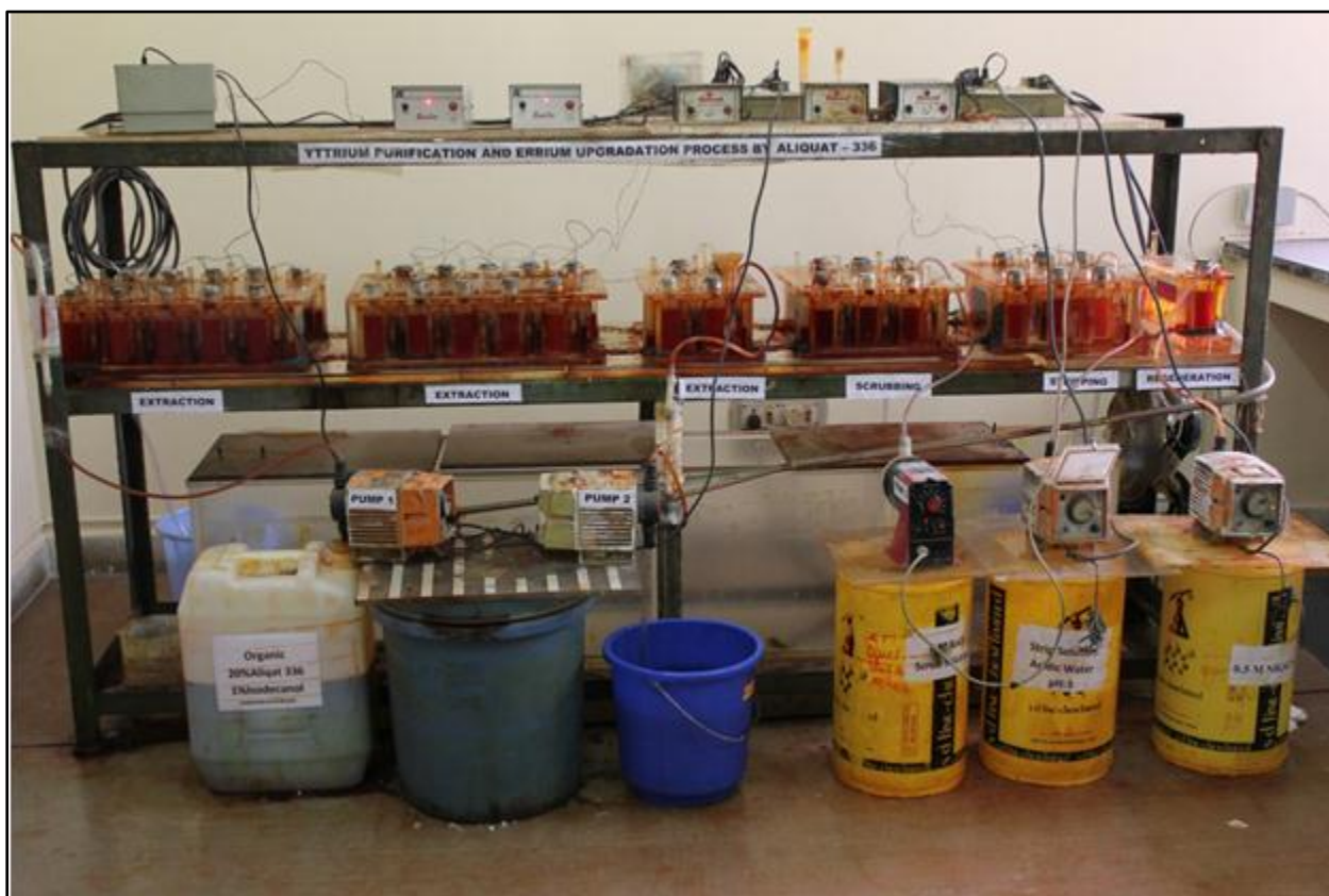
Fig. 1.5 Solvent Extraction: Mixer-Settler Assembly for Yttrium Purification
