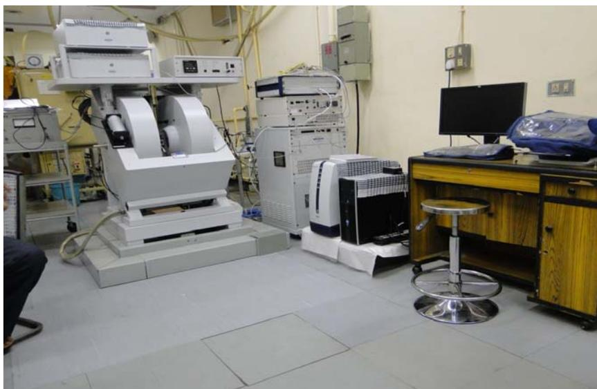
Figure 2.18: Photograph of Bruker ESP-300 EPR spectrometer
