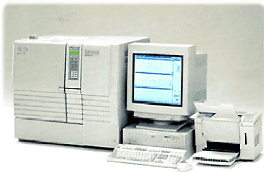
**Figure 2.5: GC-MS spectrometer**
