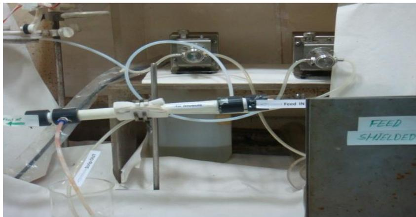
**Figure 2.11: Separation of  $^{137}\text{Cs}$  from 100 times diluted HLLW using a hollow fiber contactor**
