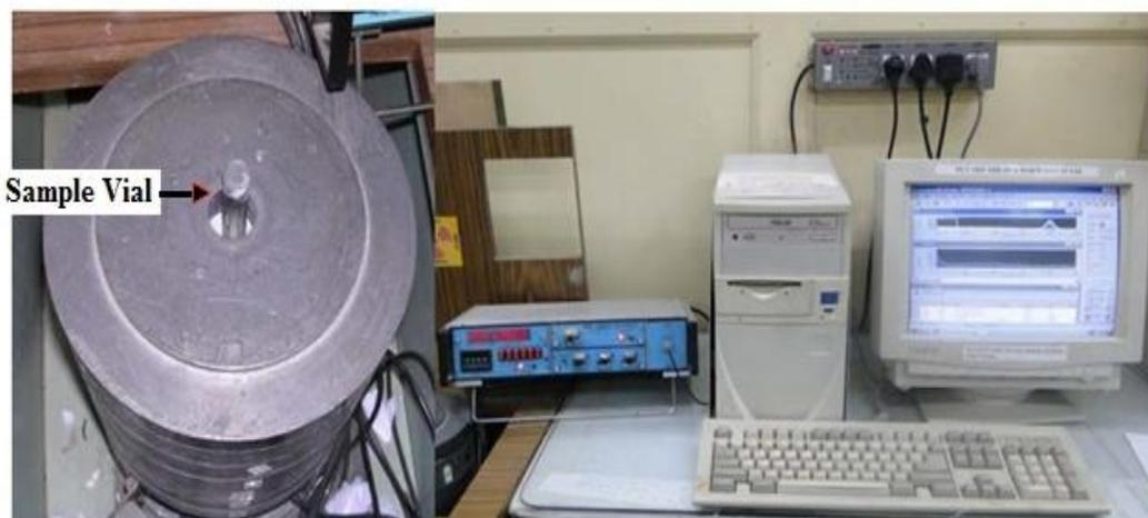
**Figure 2.2: NaI(Tl) detector used for gamma counting**
