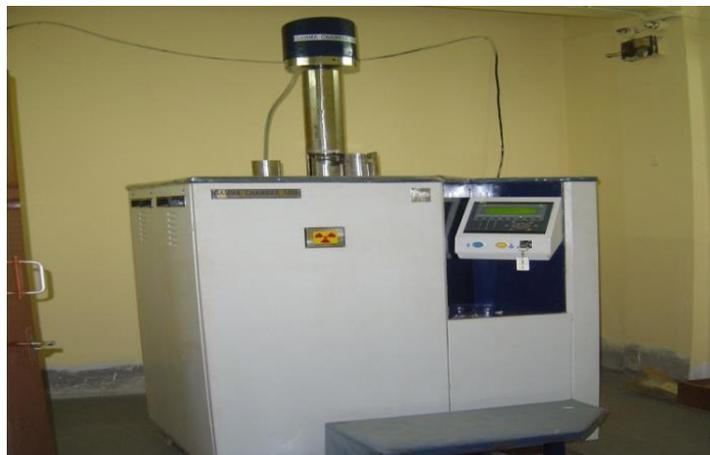
**Figure 2.7:**  $^{60}\text{Co}$  Gamma irradiation chamber
