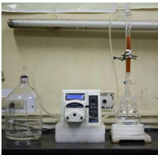
**Figure 2.5: Photograph of the experimental setup used for  $\text{LiOH}$  preparation**
