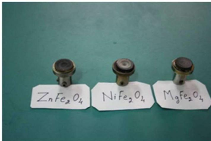
**Figure 2.4: Photograph of the target holders**
