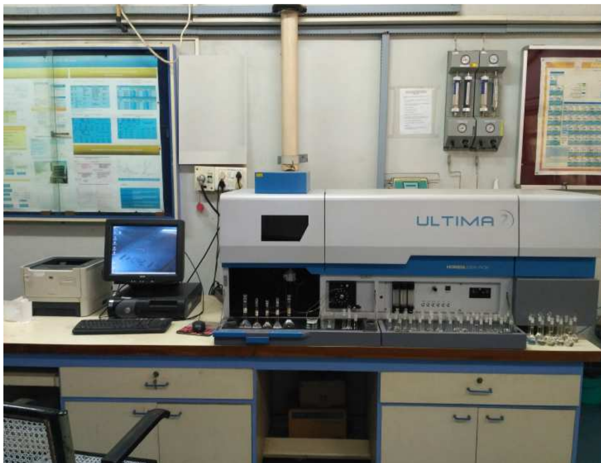
Fig.2.8. Overview of a Basic Inductively Coupled Plasma—Atomic Emission Spectrometry (ICP-AES) (EMAS laboratory)
