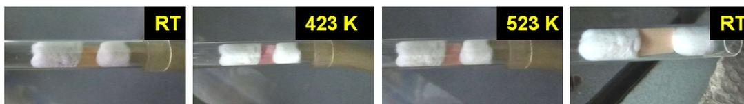
**Fig. 6.10. Estimation of pH of vapours evolved during heating of glycine-Th(IV)-nitrate gel. Gel was heated inside quartz tube and vapours were carried up to pH paper by argon gas flow**
