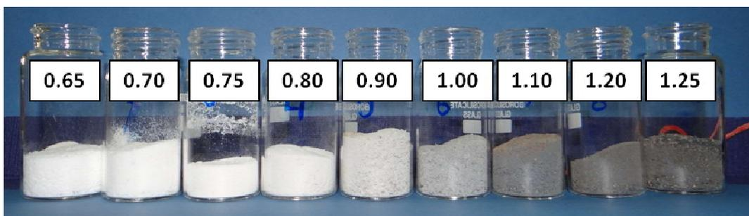
**Fig. 6.22. Photograph of as-combusted powders with varying F:O ( $0.65 \leq \text{F:O} \leq 1.25$ )**
