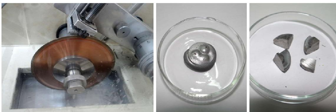
**Fig. 2.3. Metal cutting by diamond impregnated blade. Th-U alloys cut into small pieces**
