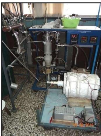
**Fig. 2.2. Vacuum sintering furnace for metal powder compacts**
