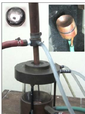
**Fig. 2.4. Photograph of Arc melting setup. Insets show copper anode cup (right frame) and as-melted alloy button (left frame)**
