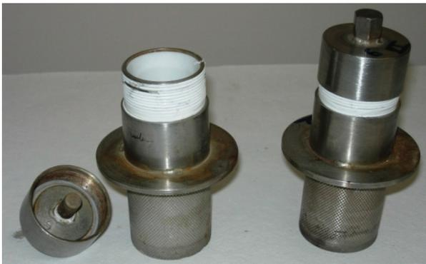
**Fig. 2.12:** Teflon-lined stainless-steel container used in leaching study.
