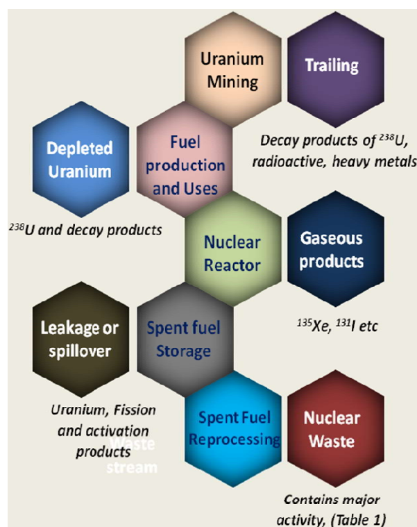
Fig. 1.1. Different stages in the nuclear fuel cycle and its associated waste.
