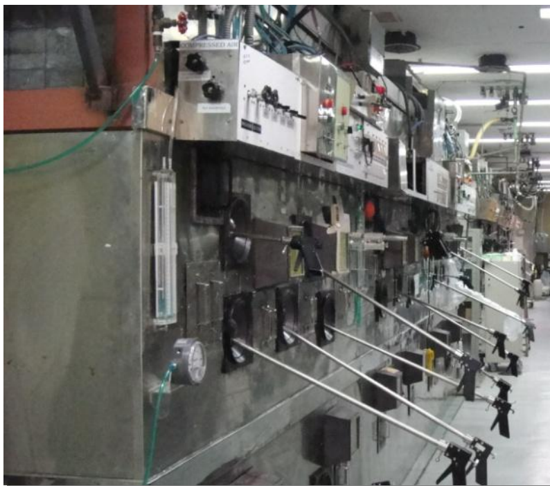
Fig. 2B.1: Photographic image of 150 mm lead shielded radiochemical processing plant
