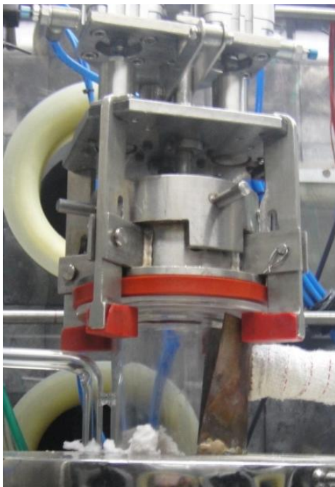
Fig. 2B.4: Semi-automated flange lid holder (photographic image of actual unit)
