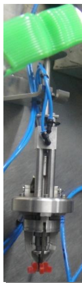
Fig. 2B.3: Semi-automatic crucible holder (photographic image of actual unit)
