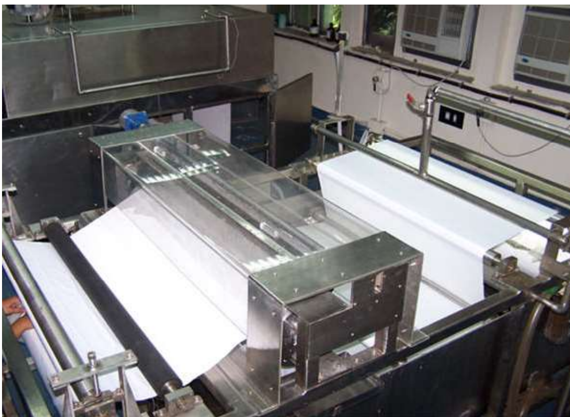
Figure 2.2: Laboratory facility for preparation of asymmetric membranes by continuous casting machine.
