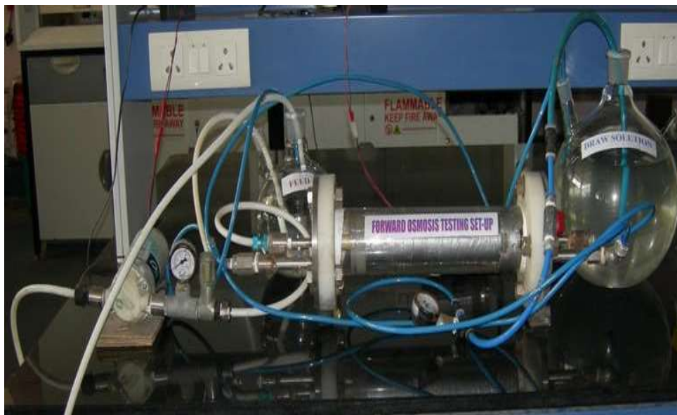
Figure 2.15: Laboratory facility for testing of FO membranes in spiral module.
