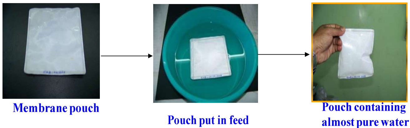
Figure 3.8a: Membrane pouch used as FO device for concentration of simulated ADU filtrate (CA membrane used).
