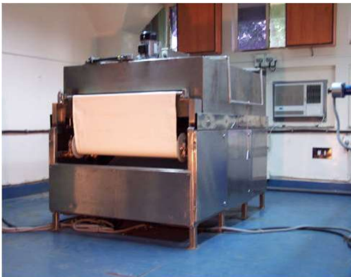
Figure 2.5: Laboratory facility for preparation of long sheet TFCPA membranes by coating machine.
