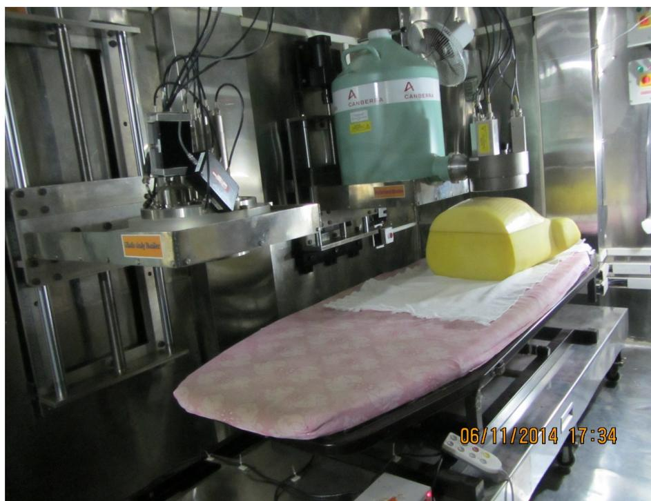
FIGURE 3.1: Actinide monitoring system, consists of an array of three HPGe detectors placed above lungs of the LLNL phantom inside totally shielded steel room.
