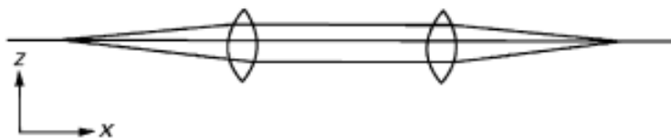
Fig. 2.3. Ion transmission due to Z- focusing
