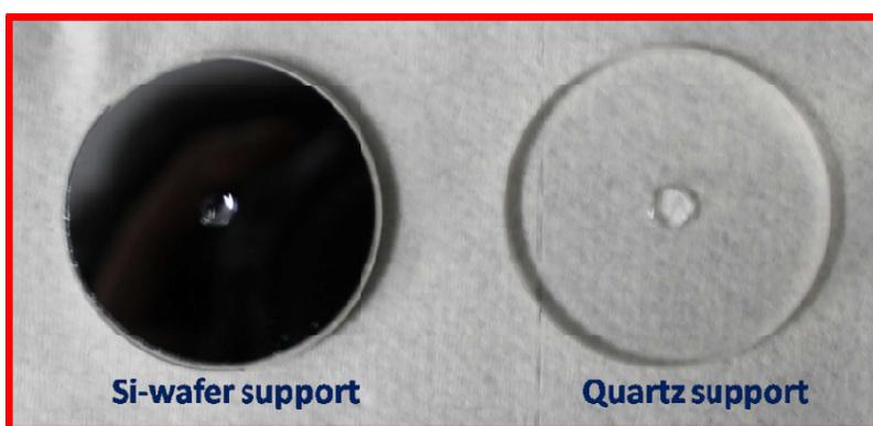
**Figure 3.12:** TXRF specimen prepared with 5  $\mu\text{L}$  volume of fluoride sample on Si-wafer and quartz sample supports.
