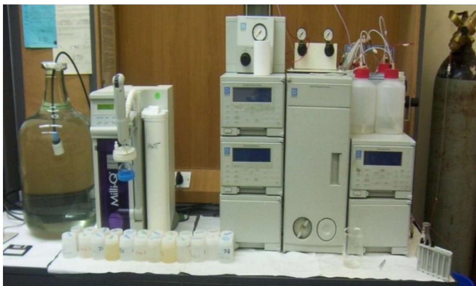
Fig. 2.2 Dionex ion chromatography system
