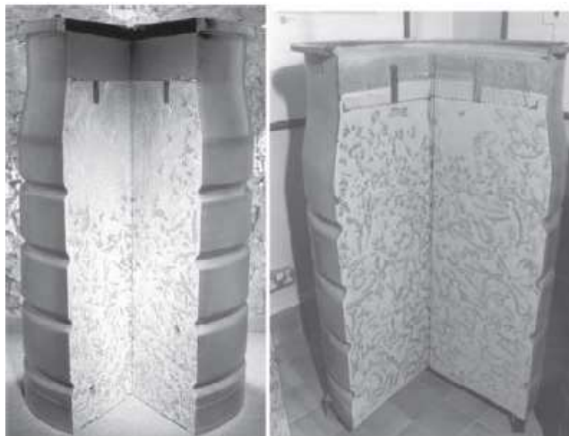
Fig. 2.2. Cement encapsulated solid, liquid and slurry LILW in 500 L drums [42]
