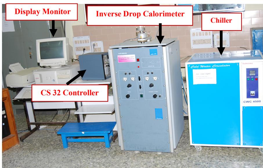
Figure 2.3 The experimental set up of drop calorimeter
