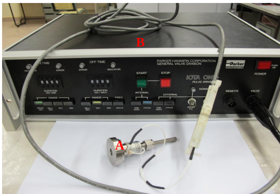
Fig. 2.5 – Photograph showing (A) Supersonic jet source and (B) Power supply.
