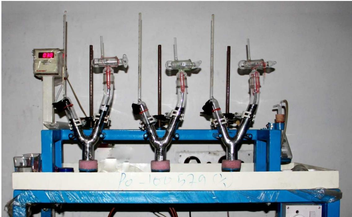
Fig. 3.14 Mercury apparatus used for  $H_D$  measurement
