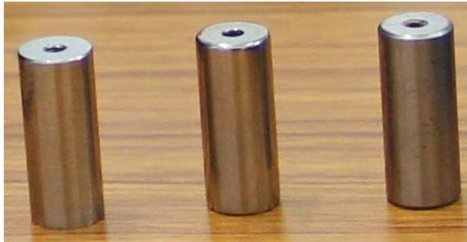
Fig. 3.17 Photograph of specimen for hydrogen charging
