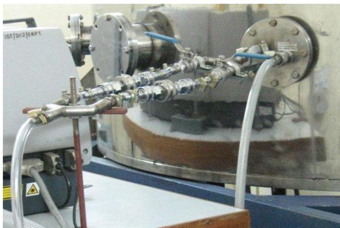
**Fig.VI.2.** Photograph of the dual filter paper sampling system.
