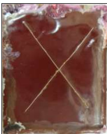
Figure 7.5: Photographs of the Epoxy Nanocontainer Coating (ENC) after 2000 h of exposure to neutral salt spray test
