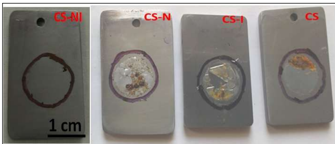
Figure 6.22: Optical photographs of the coated specimens after 1 week of immersion in 0.05 M NaCl solution. The drawn circles indicate the exposed area of the coatings.
