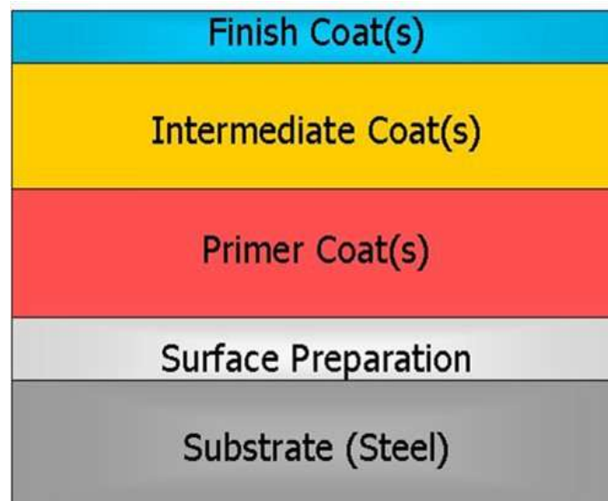
Figure 1.5: A typical coating system for marine and industrial applications
