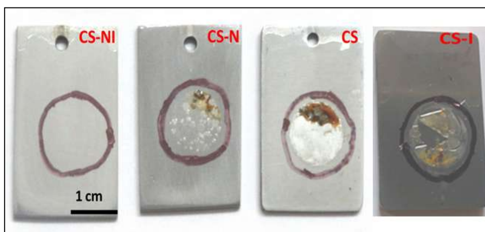
Figure 4.12: Optical photographs of the coated samples after 1 week of immersion in 0.05 M NaCl solution. The drawn circles indicate the exposed area of the coatings
