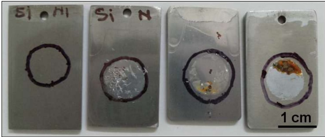
Figure 5.14: Photographs of the coated samples after 1 week of immersion in 0.05 M NaCl solution. The drawn circles indicate the exposed area of the coatings
