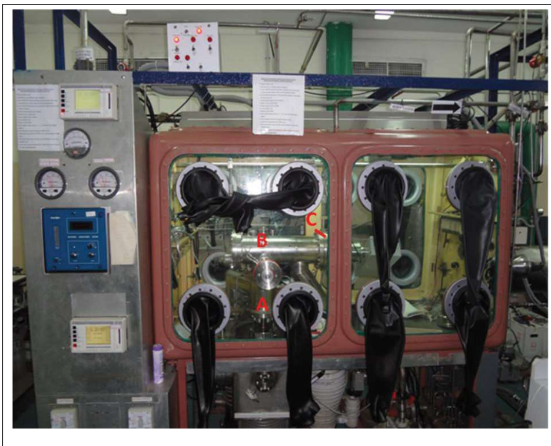
Fig.3.2. Photograph of KEMS facility inside the glove box
