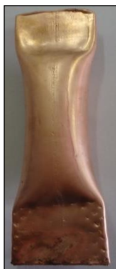
Fig. 3.6 Cu tube sealed under argon atmosphere with sample inside
