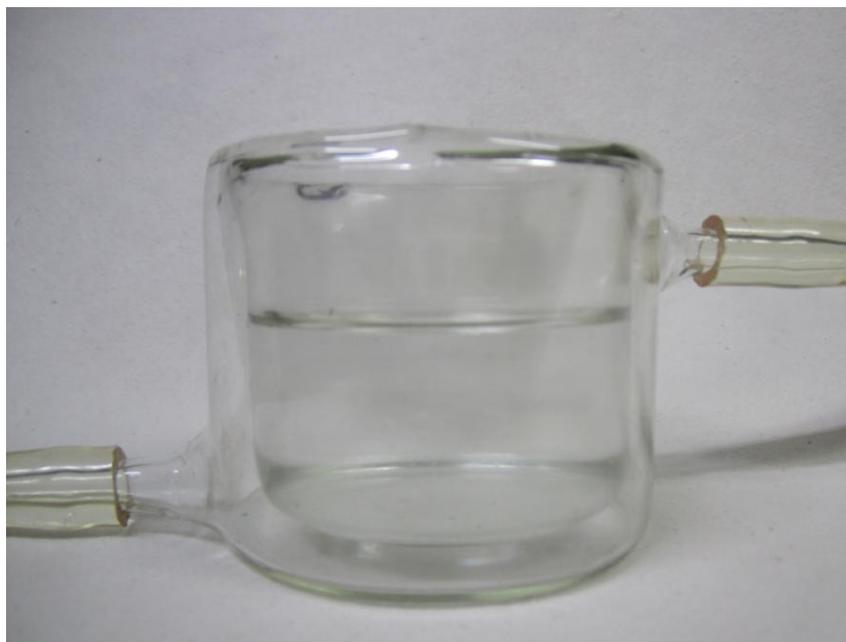
*Fig. 2.4: Double walled vessel used for solvent extraction experiments.*
