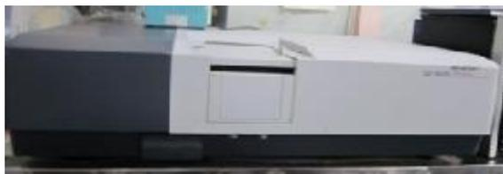
*Fig. 2.2: UV-Visible-NIR spectrophotometer (SHIMADZU UV-3600 model).*
