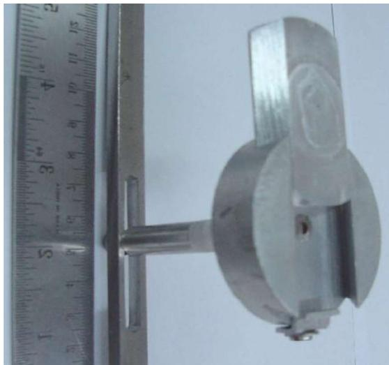
Fig. 2B.3 Photograph of the Al sample holder with a dow tail cutting groove for the sample plate
