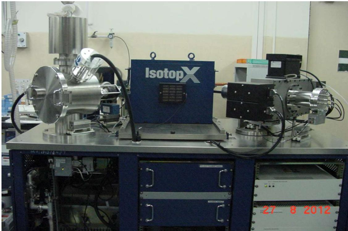
Fig. 3.1 Photograph of the TIMS instrument used for the present study
