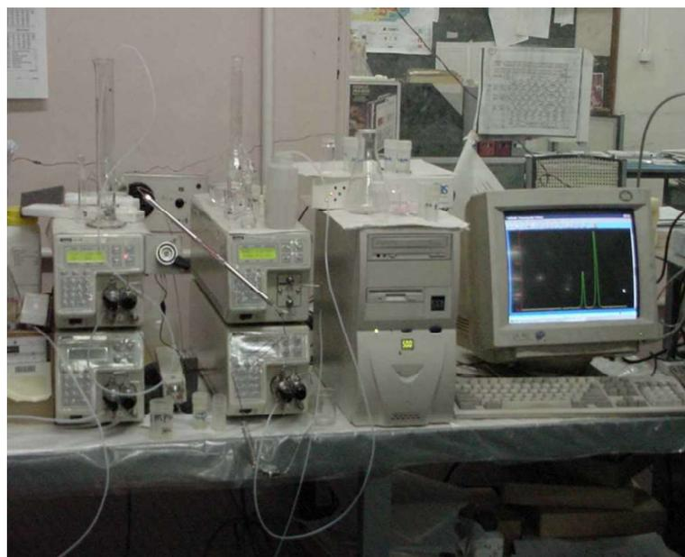
Fig. 4.3 Photograph of the components of HPLC system kept outside the fume hood.
