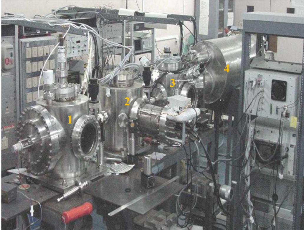
Fig. 2B.2 Photograph of the in- house developed Laser ionization- Time of flight mass spectrometer facility (1- PLD chamber, 2- QMS chamber, 3- sample chamber, 4- TOF drift tube)
