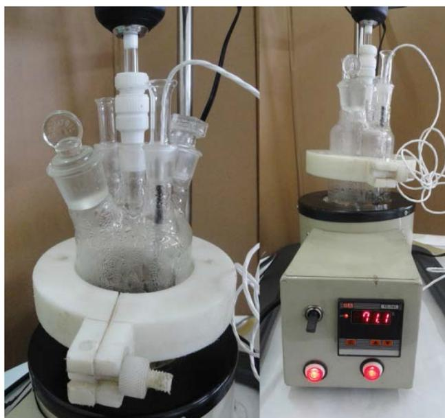
**Fig. 5.4. Glass bubble dissolver with air sparging**
