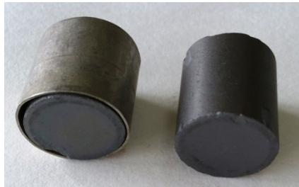
In the case of processing the spent fuel by chop leach process, the chopped fuel pins would contain the fuel covered by the SS clad along its curved surfaces. It is open only along the two circular (or oblique/elliptical to be precise) faces. Hence in all the experiments pertaining to this thesis work, the curved surfaces of the pellets are covered using a SS sheet to simulate the presence of clad during the dissolution experiments.
