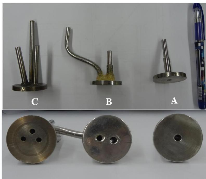
**Figure 2.2:** Photograph showing various nozzles used for the deposition of the gas sample. A) Single jet B) Double jet C) Triple jet
