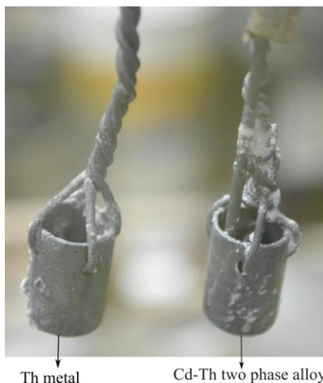
*Figure 2.11 Electrode assembly used in emf study of Cd-Th alloys.*
