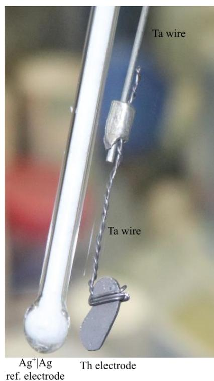
*Figure 2.10 Electrode assembly used in emf study of ThCl<sub>4</sub> in LiCl-KCl eutectic melt.*
