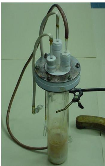
*Figure 2.3 Photograph of chlorination set-up made of quartz vessel and teflon flanges.*
