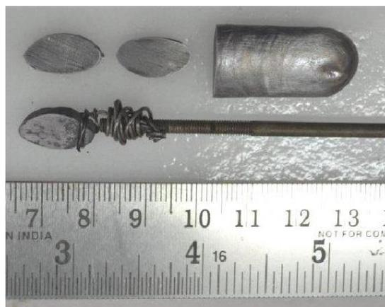
*Figure 2.8 Thorium electrode used in the present work.*
