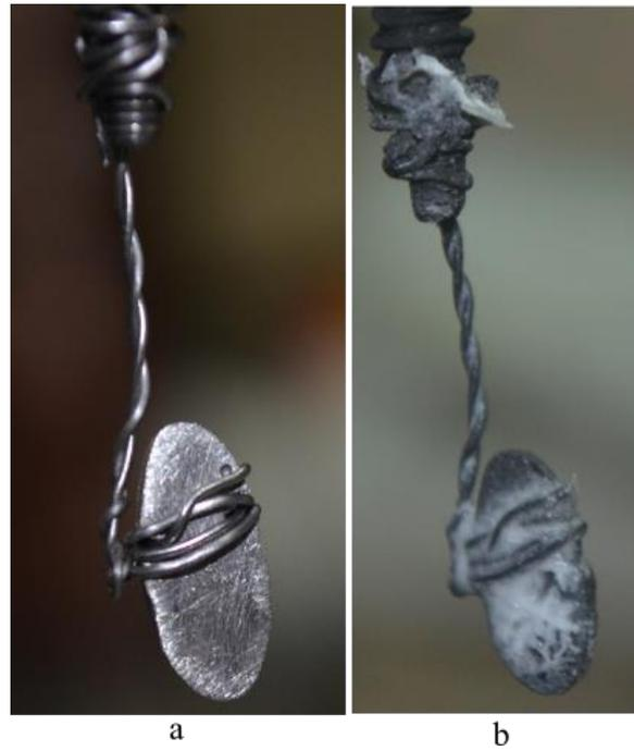
*Figure 3.21 Th electrode prepared for experiment (a) before immersion in the melt and (b) after immersion in the melt.*
