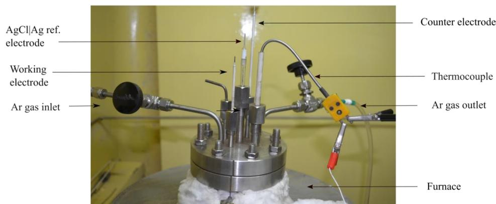
*Figure 2.13 Photograph of electrochemical cell loaded with electrodes.*
