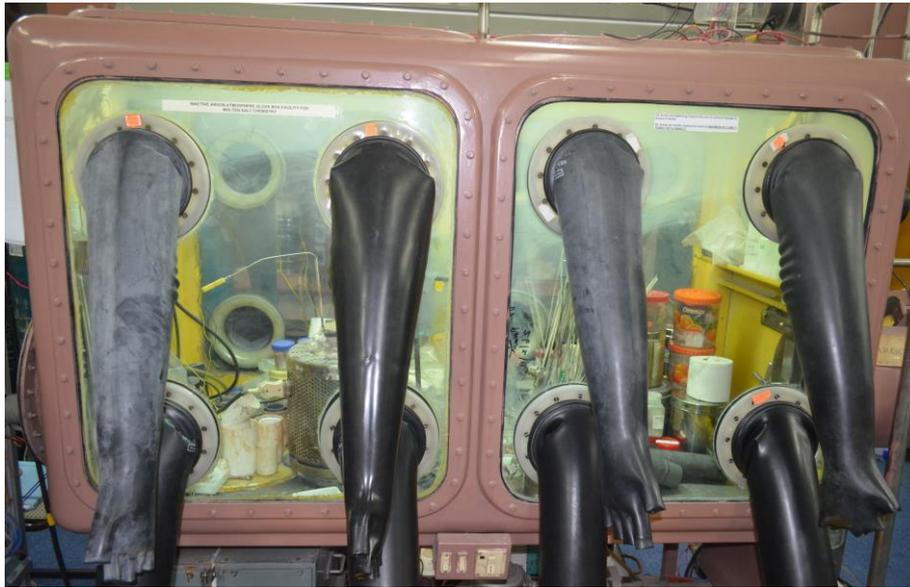
*Figure 2.2 Photograph of argon atmosphere glove box used for carrying out experiments.*
