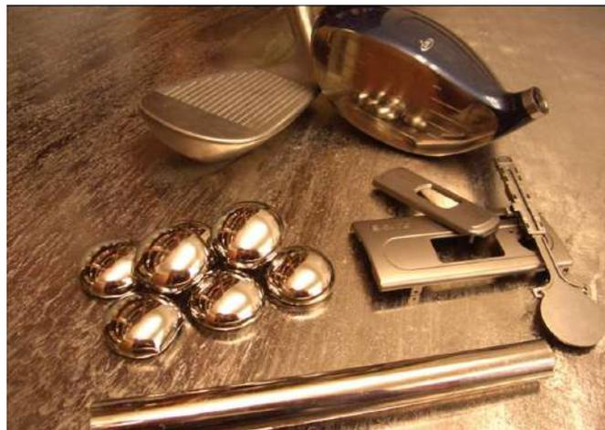
Fig. 1.2 Images of the Vitreloy bulk metallic glass hardware, including golf clubs, electronic casings, optical hardware, ingots, 12 mm diameter rod, and large plate (under the samples). Hardware courtesy of Liquid metal Technologies [18].
