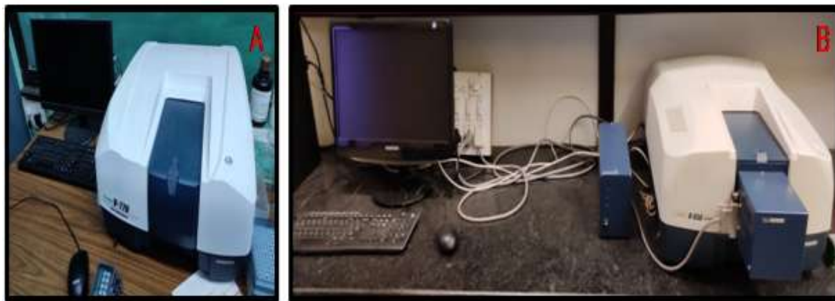
Figure 2.1: (A) JASCO V-770 UV-Vis-NIR spectrophotometer with spectral range 190-3200 nm, (B) JASCO V-650 UV-Vis spectrometer fitted with Peltier for temperature-dependent study with spectral range 190-900 nm.
