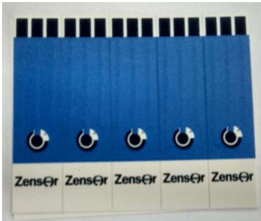
Figure 8.3: A panel of screen-printed electrode use for impedimetric assay.
