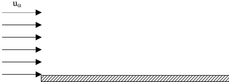
Figure 4.3 External flow over a flat plate
