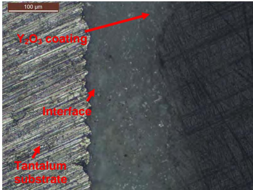
Figure 7.13 Typical optical micrograph of cross-sectional view of tantalum /yttria coating interface (as coated)
