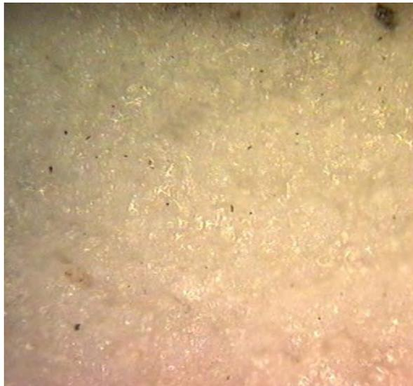
Figure 7.4. Ytria coating on tantalum rectangular token, as coated surface micrograph at 100X
