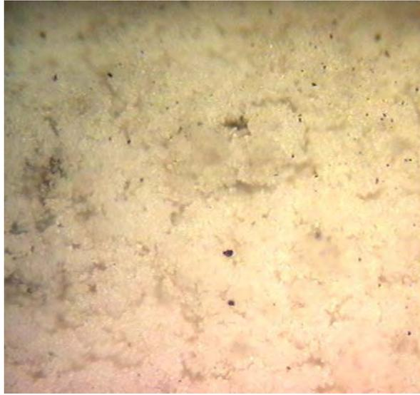
Figure 7.3. Ytria coating on tantalum rectangular token, as coated surface micrograph at 100X
