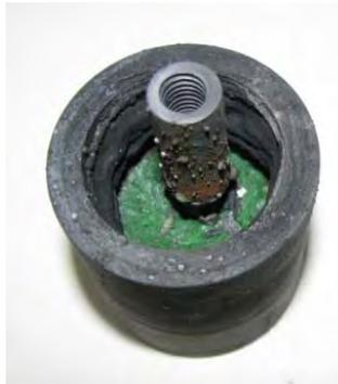
Figure 6.8 Photograph of S80 cell after the electrolysis with anode power holder embedded
