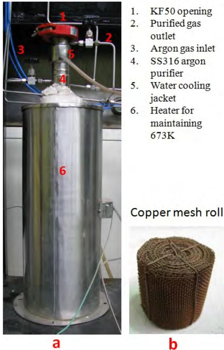
Figure 3.1 (a) Photograph of the argon purifier to generate argon with < 0.1ppm oxygen (b) Copper mesh roll absorber used in purifier
