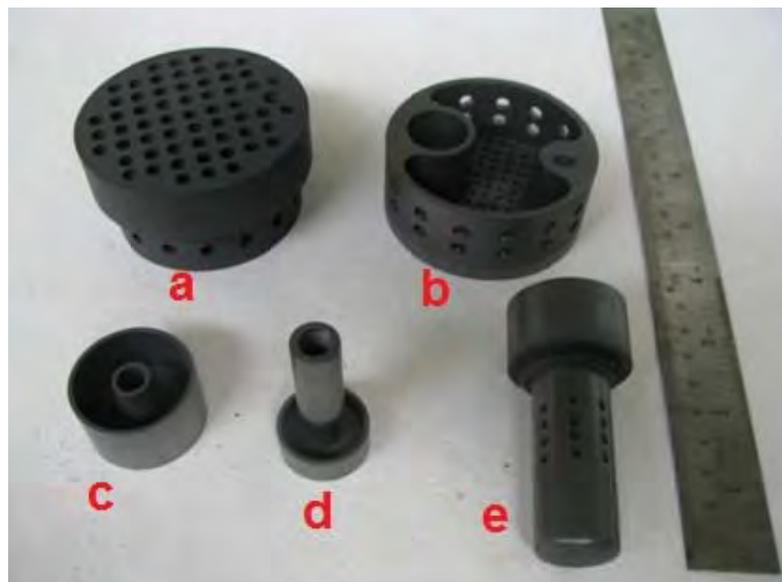
Figure 6.6 Photograph of different anodes of graphite used in the electrolysis experiment
