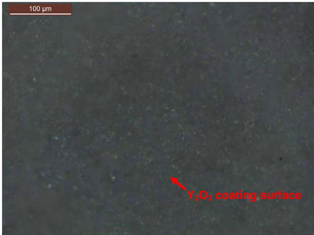
Figure 7.11 Typical optical micrograph of surface of yttria coating on tantalum substrate (as coated)
